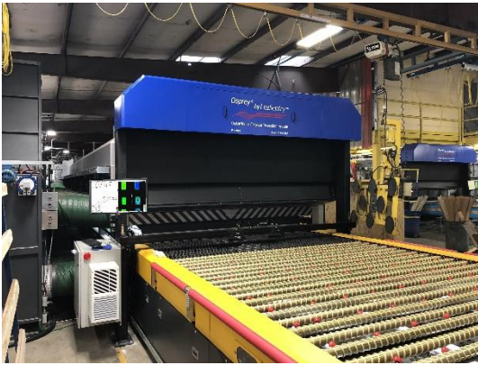
Figure 5: Example of online digital imaging method to measure optical distortion, the LiteSentry Osprey system. Photo courtesy of LiteSentry-SoftSolution.
