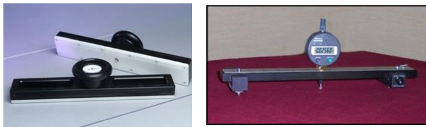
Figure 4: Surface contact gauges: flat-bottom (left) and three-point contact gauge (right)
